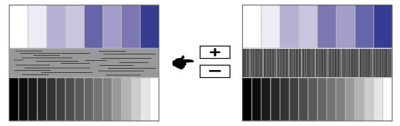
G Select "Position" in the Adjustment Program and adjust the V-Position and H-Position so that the frame of cross-hatch pattern fits into the display area.
